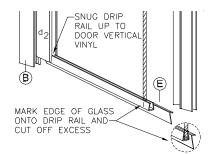
figure 5 Snug Drip Rail up against the vertical Vinyl, then cut off the excess as shown in figure.
