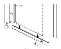
figure 4 Insert Drip Rail unto bottom edge of glass
